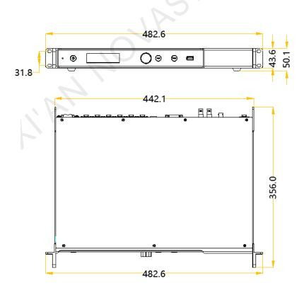
Tolerance: ±0.3 Unit: mm
