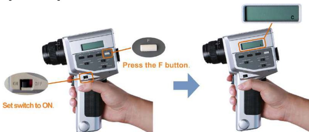
Figure 12-7 Setting CS-100A colorimeter
