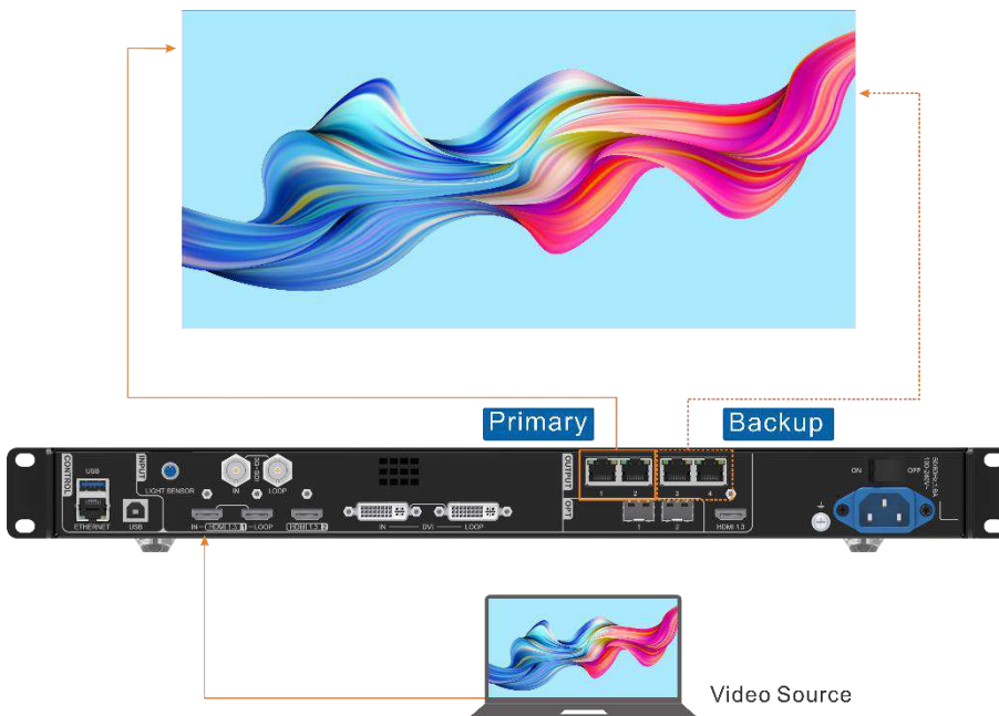
Figure 5-27 Ethernet port backup connection
